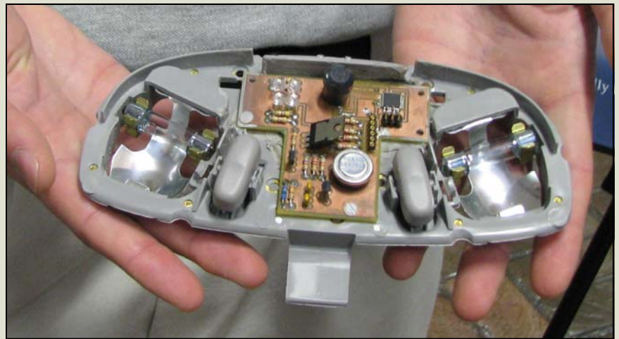
Above is the final prototype of the heat detection system.
